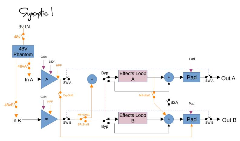
=> Oranges switches are internal jumpers or switches.
