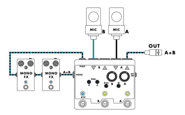
This is the same configuration as the one mono loop case, but both mics are turned on at the same time. The mix is available either on A or B outputs:
