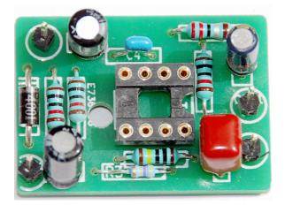
Solder the components on the PCBs, beginning by the smaller:
