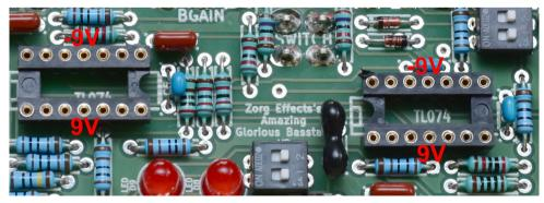
Step 4: insert the TL074 in socket U2 and the TLE2074 in socket U3.
