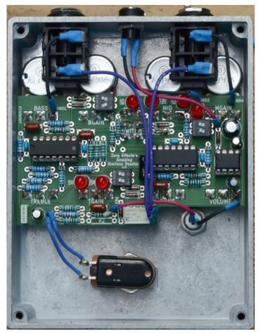
9V1 goes to +9v of the DC jack (long leg if you wish to wire it center negative) Gnd2 goes to gnd of the DC jack (short leg if you wish to wire it center negative)
