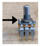
If you have un-insulated pots, stick 16mm length of window insulator under each pot of the first row. It's in order to prevent solders on the board to connect with the body of the pot and shortcut some circuits.
