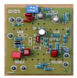
For the full Ge version, you'll notice papers on the transistors with two numbers. Susbstract the smaller number from the bigger, this will give you the transistor gain. Put the transistor with the smaller gain in Q1.
