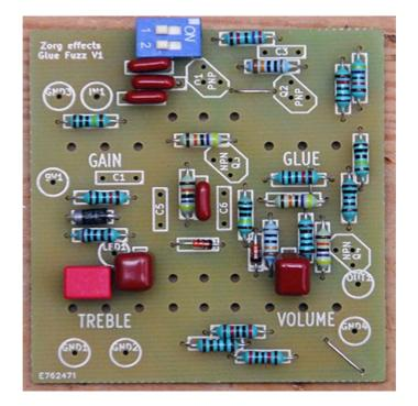
Cut the DIP14 in line socket to make soldering terminals for inputs/outputs (GND1,2,3, IN1 etc...). Then put the transistors:
