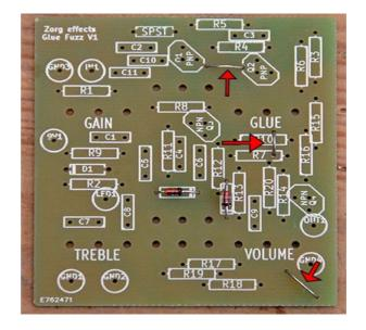
Then we're going to solder components from the smaller to the taller. First, diodes and resistances. You shall take care of the diodes positions. They MUST be on the same direction as on this picture :
