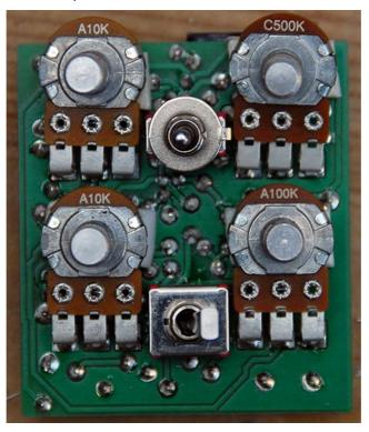
Soldering the switch is a bit shitty. First you should push it all the way into the board. If you let some space between the board and the switch, the problem will be that the height of the switch will be a bit higher than the pots height and this can somewhat be a problem when screwing the pots on the enclosure...
