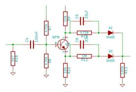
To produce the octavia fuzz sound you can use an audio transformer and a pair of diodes, or the schematic above.
