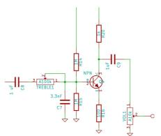
C8 is a decoupling cap, together with R15 it makes a high pass filter, cutting at F=1/(2xPixC8xR15)=15Hz.
