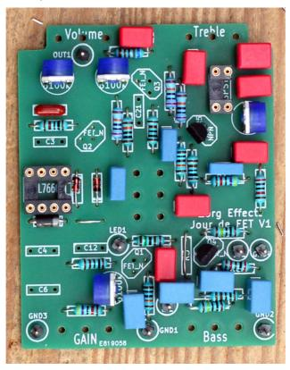
We now can add electrolytic caps. Beware of the direction of electrolytic caps, they must be with the white negative (-) stripe as shown by the arrows on the picture below.
