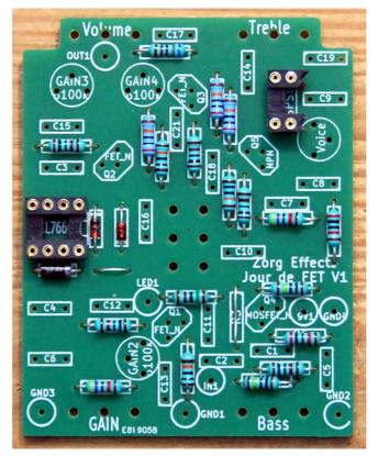
Note that on this picture above, the socket cut is far from ideal. Actually you'll need a bit of space between the socket and C14 and C9 to glue the dip switch with heat shrink tube. We'll see that point later, but for now, if its touching C14 or C9, shorten the socket a bit with pliers.
