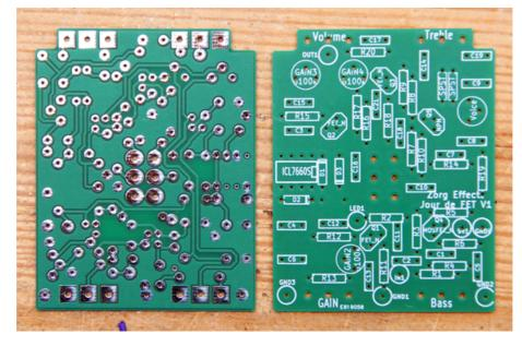
On copper side, begin by soldering the 3 J201 CMS transistors. Beware of their directions, they must be like on the picture below. The purple dot shows the pad where the transistor's grid must be soldered. The grid being the single leg on the rectangle's side. Because of the transistor's size, one must use a precise soldering iron. Be careful that the solders do not overlap eahc others. Test with your multi-meter if needed.
