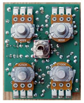
Soldering the switch is a bit shitty. First you should push it all the way into the board. If you let some space between the board and the switch, the problem will be that the height of the switch will be a bit higher than the pots height
