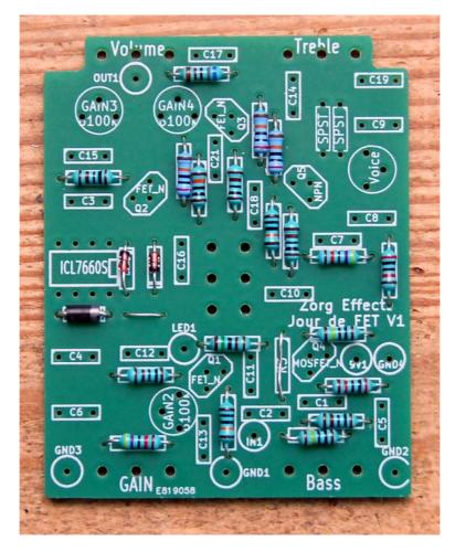
Add the sockets. The  $2^{nd}$  socket is used to level up the dip switch for easier access. You'll have to cut it in half and keep only four legs:
