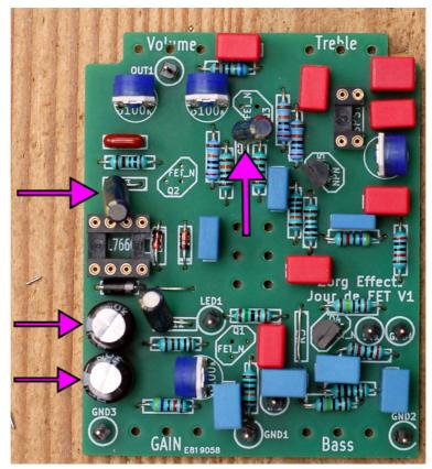
Now flip the board. We're going to solder the switch and pots on the other side. Begin with the DPDT switch and pots at the end.
