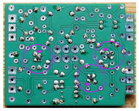
Flip the board and solder the 2 jumpers by using resistance's legs. One of the is used to bypass R3. See picture below.
