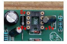
Step3: if step 2 is ok, add the ICL 7660scpa in his socket. Be careful of the orientation or you'll blow it up. Important: the pedal can work without the ICL7660s, but you'll need to re-bias it. You'll also have less gain and output volume.
