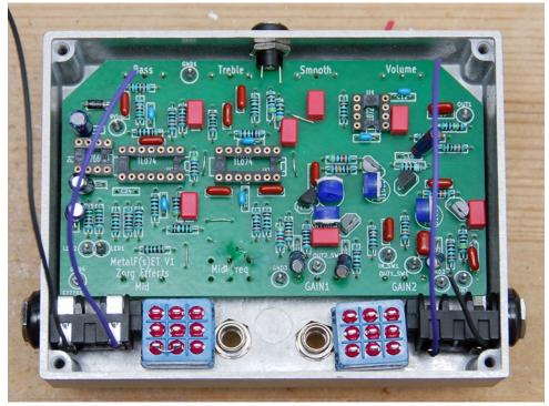
Prepare the audio jacks by removing 2-3mm of the rounded part on top of them, so that they can fit in the box. Use pliers for that. Then solder wire and heat shrink tube to the jack's legs. When it's ready, put your jacks in the box.
