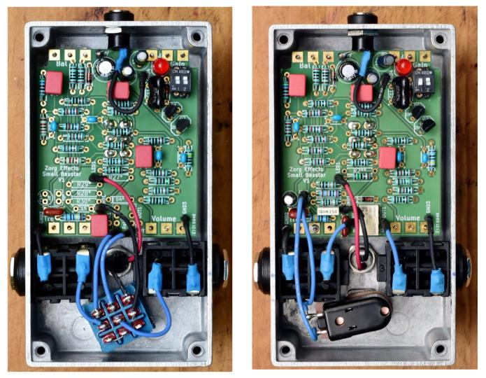
Here's what to solder in both options, it's important to use heat shrink tube to strengthen and protect your connexions (on the board and on the jacks)
