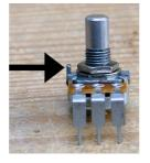
Stick 16mm length of window insulator under each pot. It's in order to prevent solders on the board to connect with the body of the pot and shortcut some circuits.
