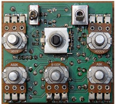
Soldering the switch is a bit shitty. First you should push it all the way into the board. If you let some space between the board and the switch, the problem will be that the height of the switch will be a bit higher than the pots height and this can somewhat be a problem when screwing the pots on the enclosure...
