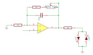
This one as a much simplifier explanation: the opamp will amplify the signal up to it's voltage rail value +/-9v. Then the leds will shortcut the signal to ground when the signal is higher than their threshold of +/-2V.
