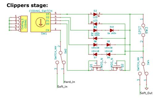
The clipping stage provides the choice between 4 different clippers. For each clippers there's the possibility to use symmetrical or asymmetrical clipping and hard or soft clipping. So there are 2\*2\*4 = 16 combinations available.
