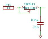
This a simple RC low pass filter to smooth the distortion. Frequency cut ranges from 1/(2xPIx(R11+TREBLE1)xC13) = 312Hz to 15915kHz.
