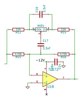
This is a mid frequency cut/boost filter. C14 is a decoupling cap. The formula to get the cut off frequency is: Assuming R13 = R15 and R14=R16  $F=(1 / 2 \times pi) \times Sqrt((2 \times R13 + MID1)/(R13 \times MID1 \times C16 \times C17 \times (R13 + R14)))$ Giving us F=760Hz for the filter center frequency.
