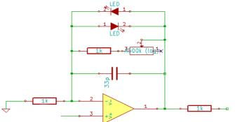
Leds will provides smooth clipping distortion. Being green leds, if the output of the opamp rise higher than their threshold (+/-2V), they will short circuit the GAIN pot and 1k resistance, but as soon as the gain pot is short circuited the gain of the
