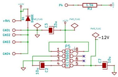
The 1N4001 D1 diode is here to prevent reverse voltage accidents.
