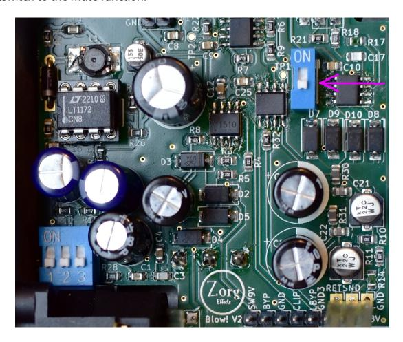
**+48V**: Power on or off the phantom supply for condenser mics. The led becomes red when it's powered on.
