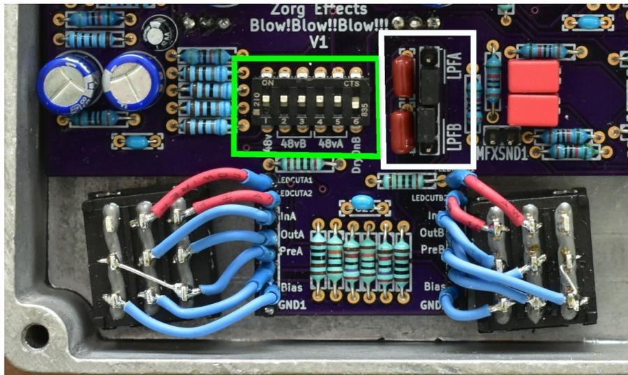
On these mini switches, the five from the left are used for phantom power. The first left labeled « 48v » is used to turn create the phantom power from the 9V. The next two switches from the left labeled « 48vB » are used to assign the phantom power to channel B and the last two labeled « 48vA » assign the phantom power to channel A.
