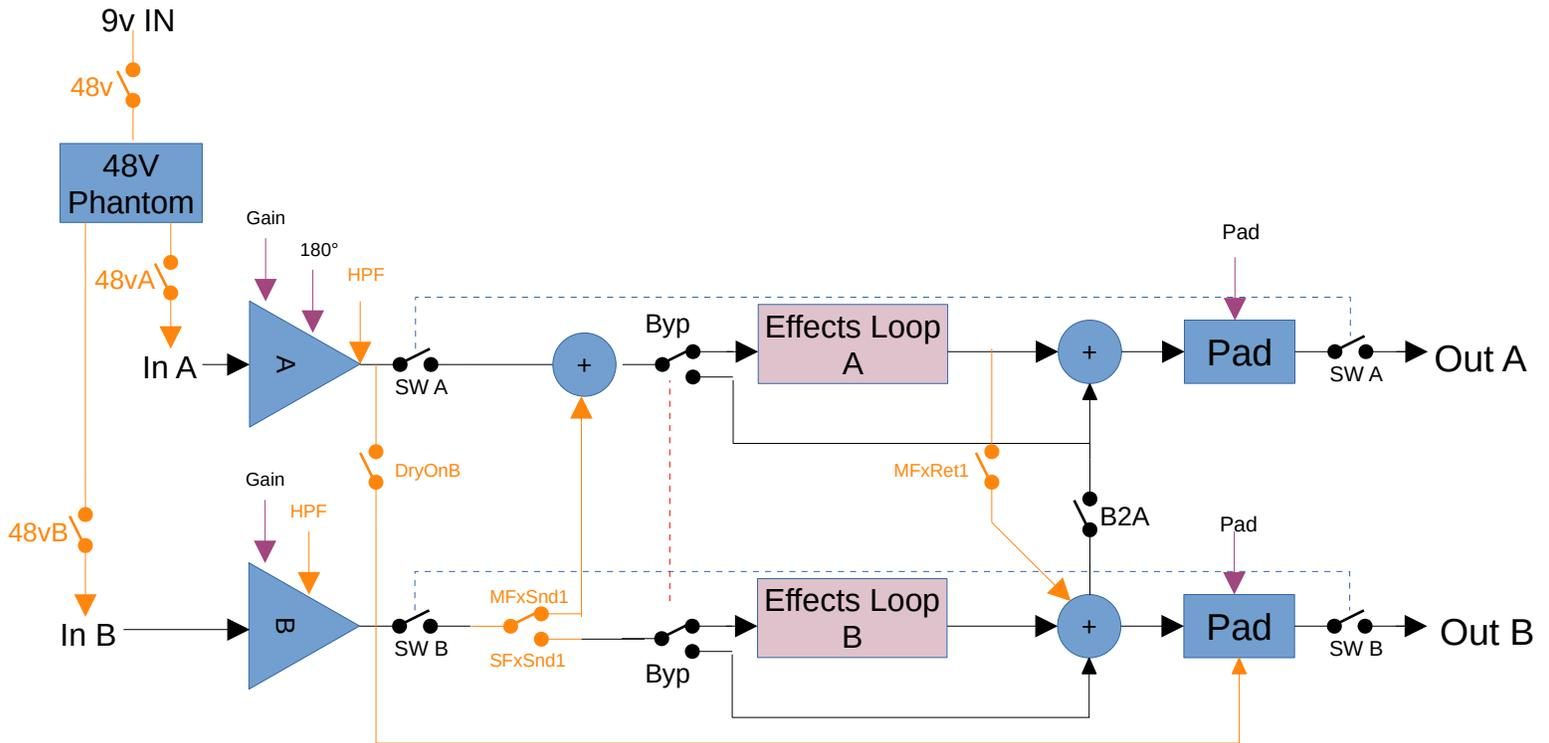
=> Oranges switches are internal jumpers or switches.
