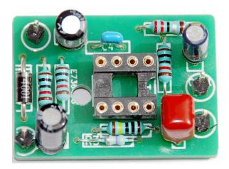
Solder the components on the PCBs, beginning by the smaller:
