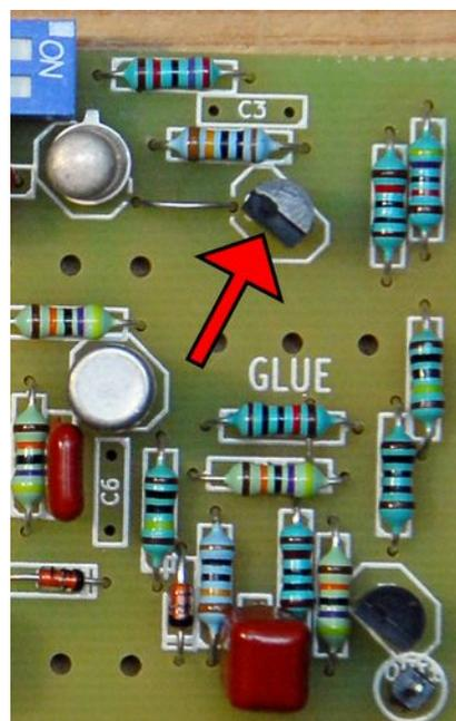
We now can add electrolytic caps. Beware of the direction of electrolytic caps, they must be with the white negative (-) stripe as shown by the arrows on the picture below. One should also tilt a bit the caps so that the box can close:
