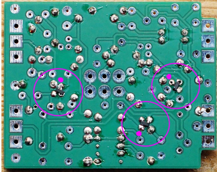
Flip the board and solder the 2 jumpers by using resistance's legs. One of the is used to bypass R3. See picture below.
