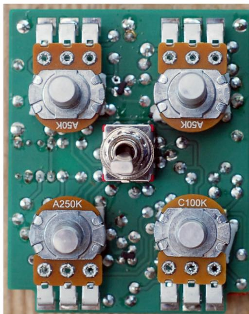
Soldering the switch is a bit shitty. First you should push it all the way into the board. If you let some space between the board and the switch, the problem will be that the height of the switch will be a bit higher than the pots height
