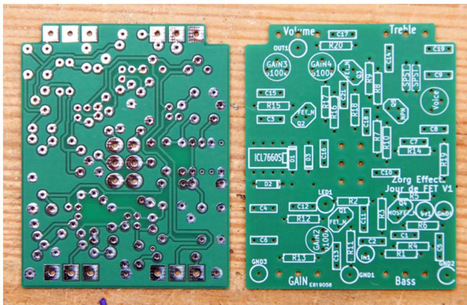
On copper side, begin by soldering the 3 J201 CMS transistors. Beware of their directions, they must be like on the picture below. The purple dot shows the pad where the transistor's grid must be soldered. The grid being the single leg on the rectangle's side. Because of the transistor's size, one must use a precise soldering iron. Be careful that the solders do not overlap each others. Test with your multi-meter if needed.
