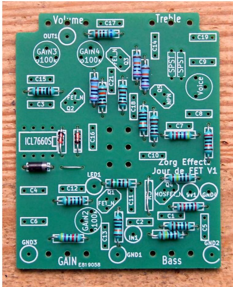
Add the sockets. The 2<sup>nd</sup> socket is used to level up the dip switch for easier access. You'll have to cut it in half and keep only four legs:
