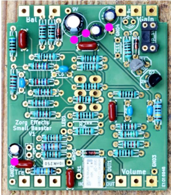
Cut the 9 in line socket to make soldering terminals for inputs/outputs (GND1,2,3, IN1 etc...). In the case of the true bypass relay option, two pins must be soldered in the sw\* print, and two others in OUT1 and IN1. Without the option, sw\* should be left empty and pins must be soldered in IN and OUT inside the relay's empty print.
