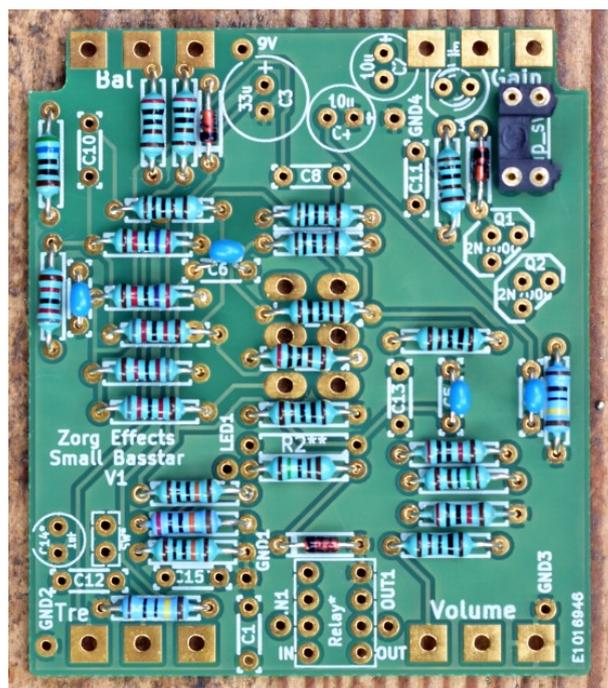
Then add the wima/panasonic/kemet caps, the transistors (beware of their directions, flat side must be has marked on the board), the optional relay and the electrolytic caps. Beware of the electrolytic caps direction. They must placed be with the white negative (-) stripe as shown by the magenta dots :
