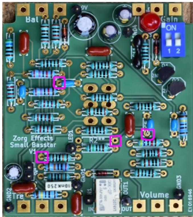
If you don't get the right tensions, check with a voltmeter that you didn't shortcut the 9v rail to the ground with a bad solder.
