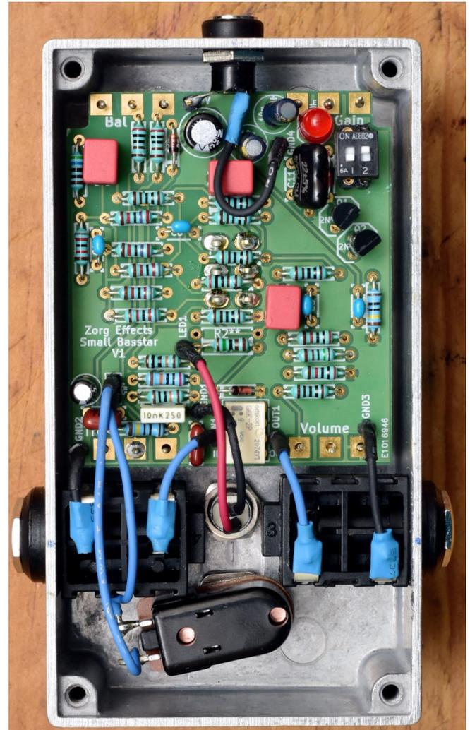
Here's what to solder in both options, it's important to use heat shrink tube to strengthen and protect your connexions (on the board and on the jacks)
