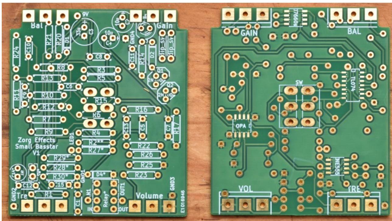
Note that it's a two side PCB. Components will be harder to unsold than on a single side PCB. Be very careful!
