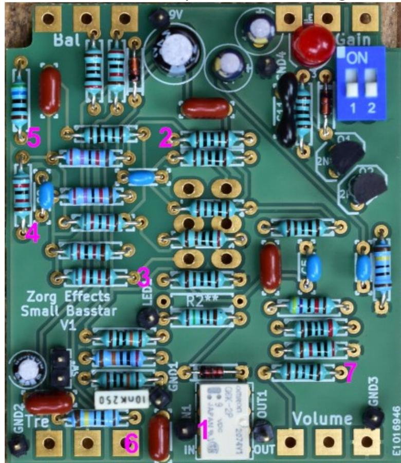
1- This is the input. No signal here might come from bad solders of the input wires.
