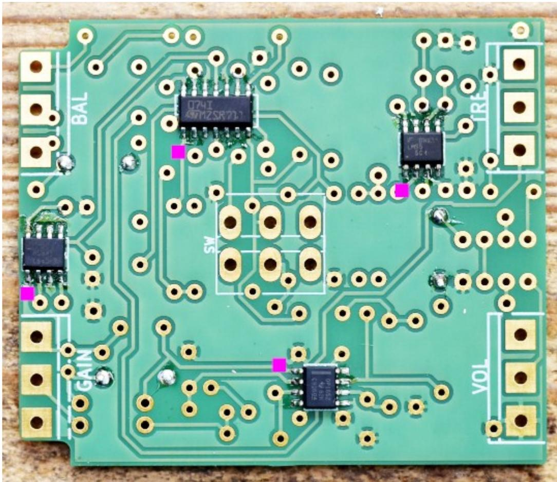
On the other side we're going to solder the components from the smaller to the bigger. First the diodes and resistance. Beware of the diodes directions. They must respect the directions shown in this picture:
