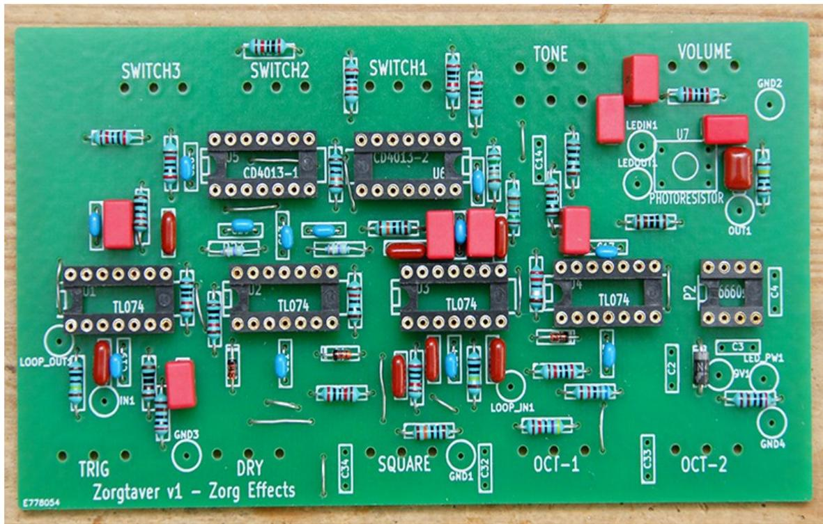
Cut the SIL12 in line socket to make soldering terminals for inputs/outputs (GND1,2,3, IN1 etc...). Then put the NSL-32 photoresistor.
